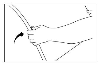
2. Remove the forward floor panel of the load floor cargo organizer and place it in the vehicle while you are removing the spare tire.
